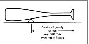
E.3.4.2 For boats first measured after 1st March 1994 the keel casting shall be weighed, measured and numbered before being fixed to the boat. The number shall be engraved on the port side at the location of the upper template, 200mm from the aft edge of the keel.
